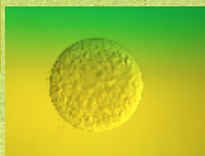
NaOH treated starch containing PVA-PAA hydrogel beads.
