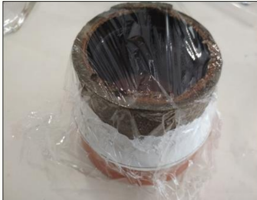
Reactor made from asbestos-cement pipe via adhesive and coverage
