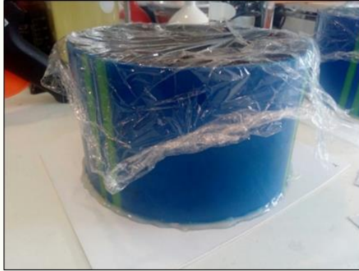
Reactor made from HDPE pipe via adhesive and coverage
