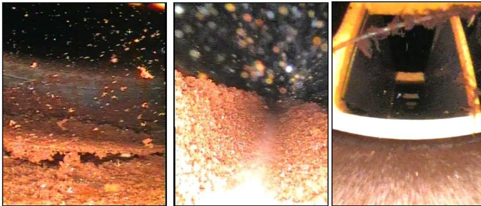
**Figure 2 – 4.** Sediment accumulated inside the DNMD (first and second picture) and the artificial substrate inserted in the special framework.
