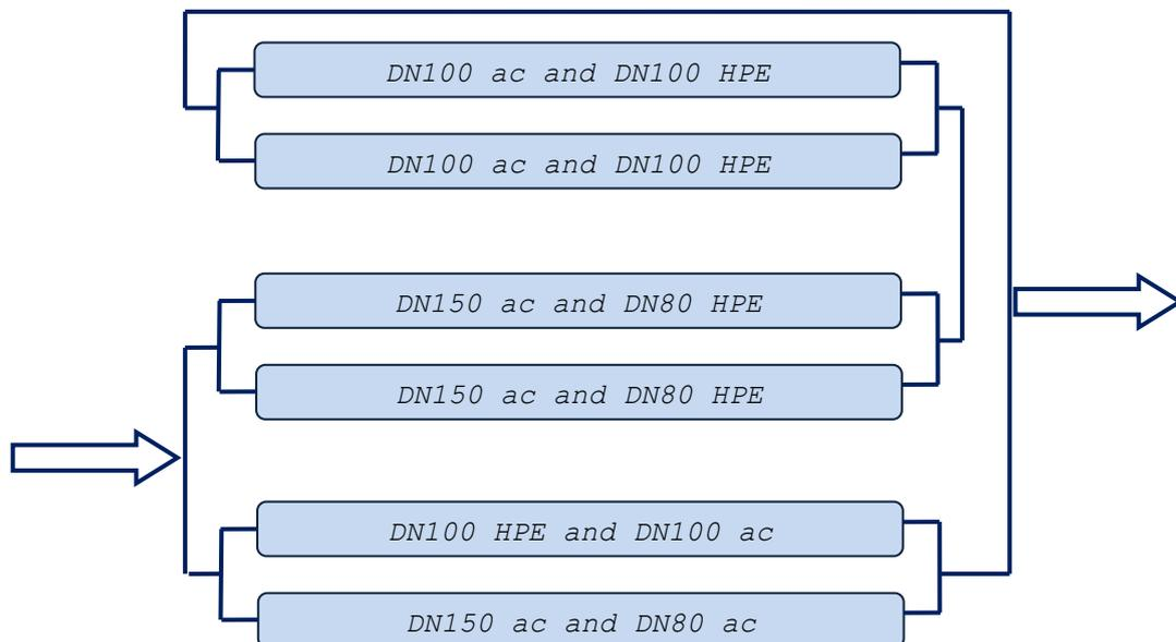
**Figure 1.** Distribution Network Model Device (DNMB) flow chart and material and diameter setup.
