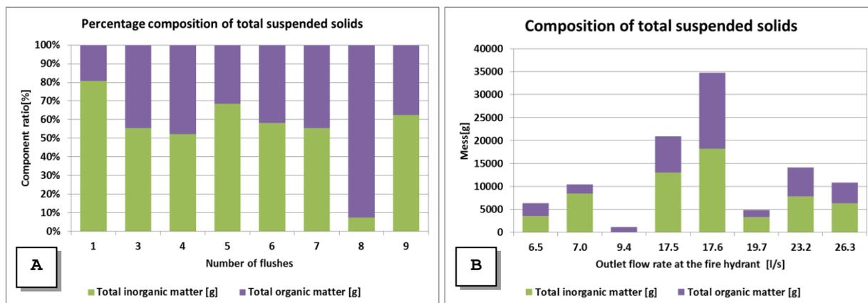
**Figure 7/A.-7/B.** Percentile composition of the flushed matter (7/A), and flushed mass and composition (7/B).
