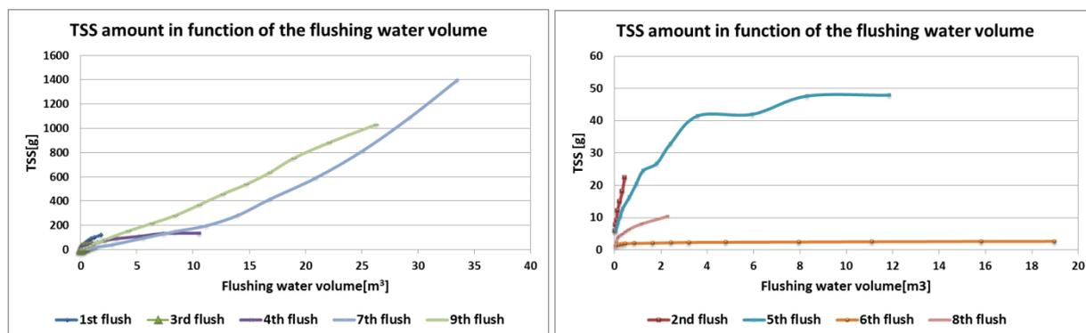
**Figure 5 - 6.** Total flushed matter as a function of the flushed water volume.
