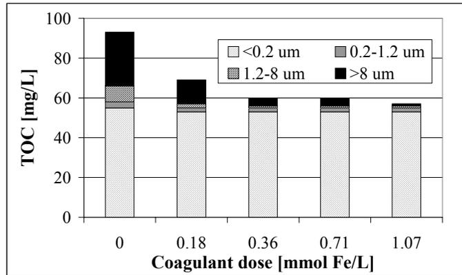
**Figure 2.** Residual TOC fractions (ferric-chloride)
