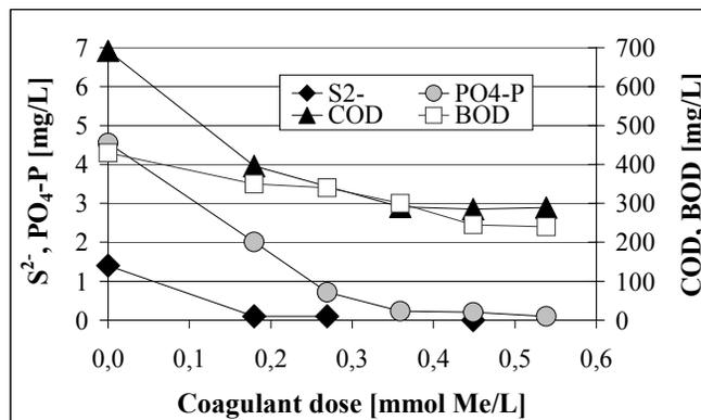
Figure 7. Residual dissolved sulphide, ortho-phosphate and organic concentration
