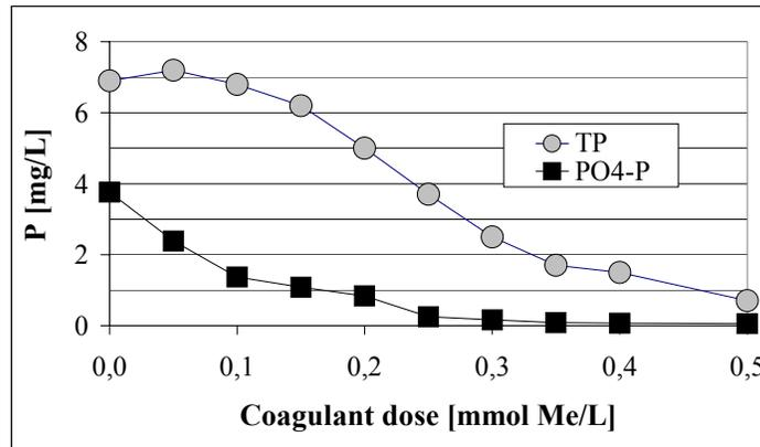
**Figure 3.** Residual TP and  $\text{PO}_4\text{-P}$  concentration (aluminium-chloride)
