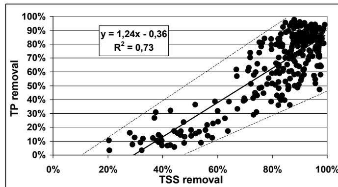
**Figure 4.** TP removal versus TSS removal
