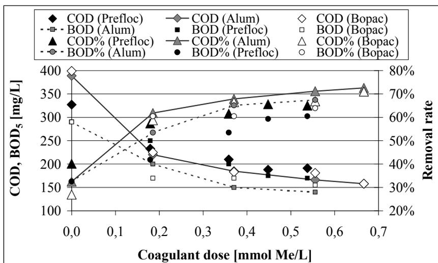
Figure 1. Removal of organic matter by feeding different coagulants
