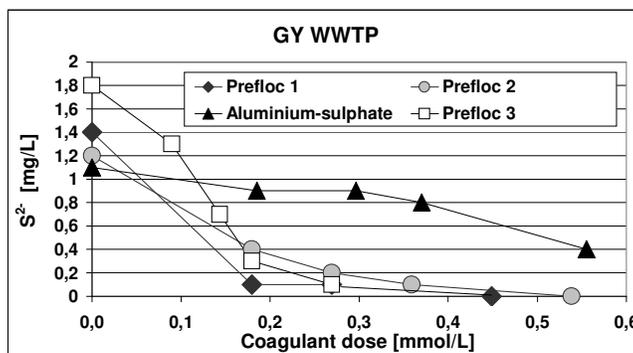
FIGURE 7. Residual dissolved sulphide concentration
