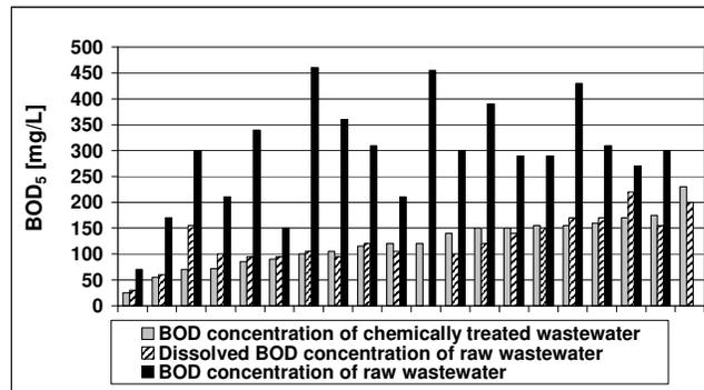
FIGURE 3. BOD<sub>5</sub> concentration in raw and coagulated wastewater
