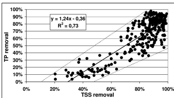
FIGURE 6. TP removal versus TSS removal
