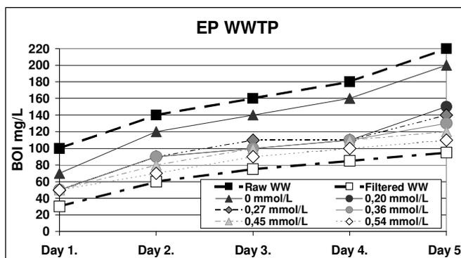
FIGURE 4. Daily BOD values in raw, filtered and chemically treated wastewater
