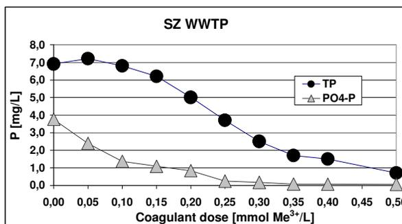
FIGURE 5. Residual TP and PO<sub>4</sub>-P concentration
