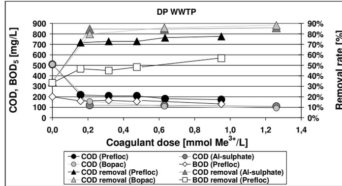
FIGURE 1. Removal of organic matter by feeding different coagulants
